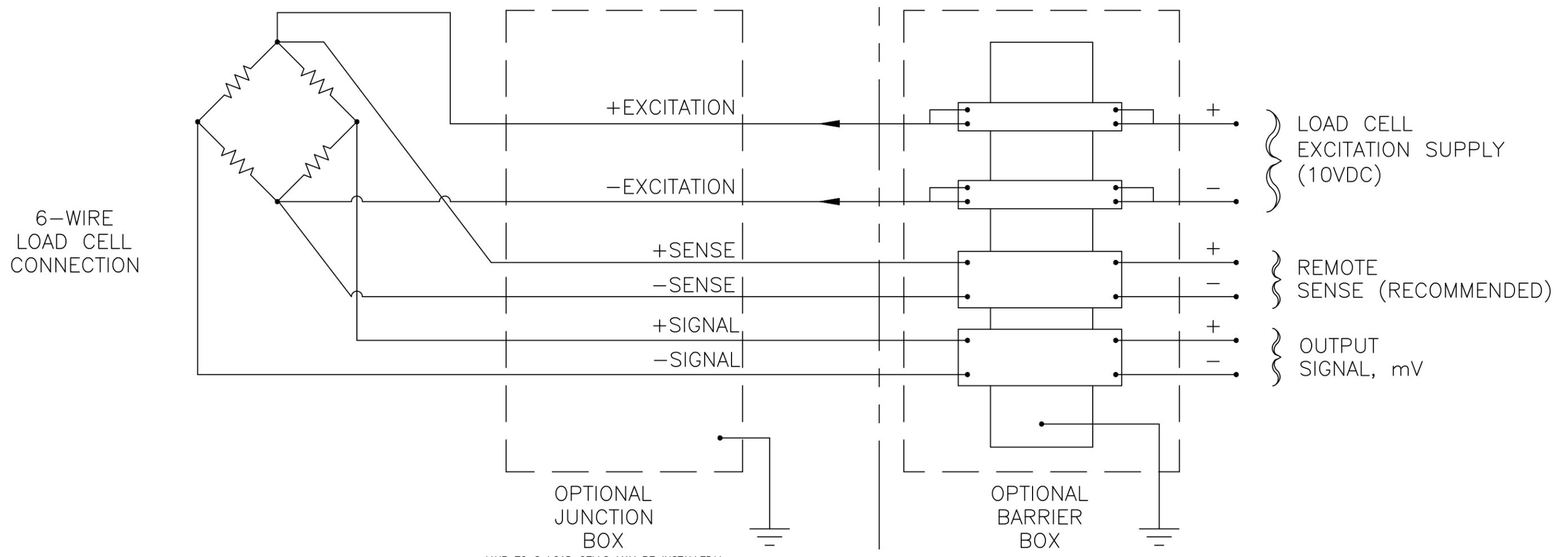
\*\*UP TO 8 LOAD CELLS MAY BE INSTALLED\*\*
